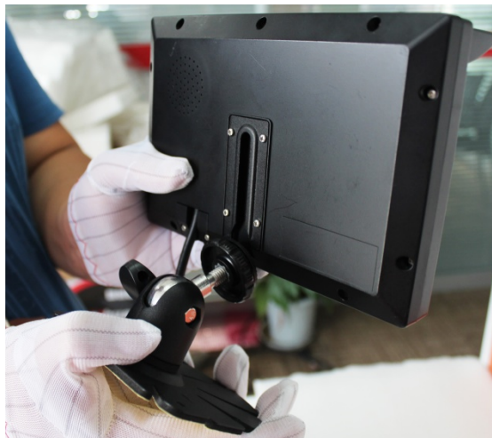
Figure 2-2 Installing bracket on the screen
