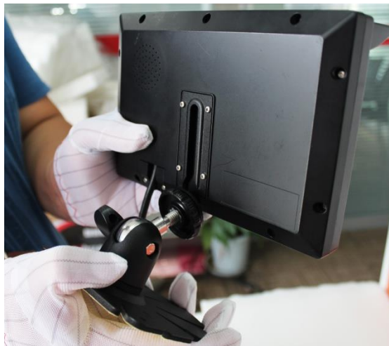
Figure 2-2 Installing bracket on the screen
