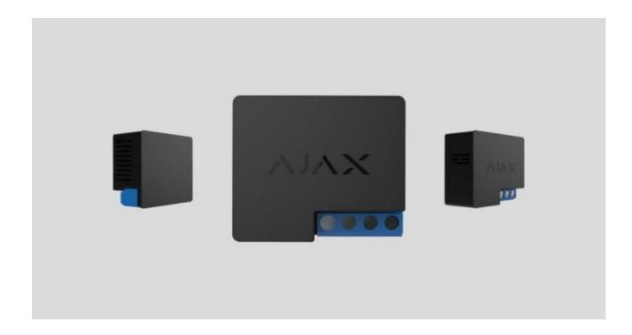
**Relay** is a wireless, low-voltage relay featuring potential-free (dry) contacts. Use Relay to remotely switch on/off appliances powered by a 7–24 V DC source. Relay can operate both in pulse and bistable mode. The device communicates with a hub via **Jeweller** radio protocol. In the line of sight, the communication distance is up to 1,000 m.
