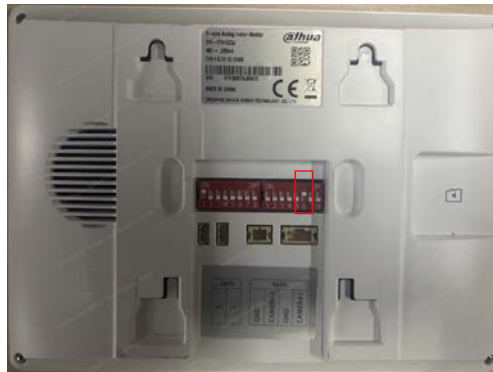
Figure 2-2 Figure 1-2 Adjust the third dip switch
