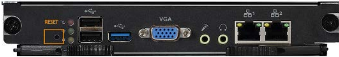
Figure 1-4 Location of RESET pinhole on M60 main control board
