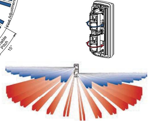
Two discrete Dual PIRs in a single housing, 2 detection areas - upper and lower can be covered respectively. Each detection direction can be moved 180 degree respectively.
