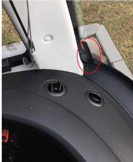
Figure 2-18 Inside installation of mobile network antenna
