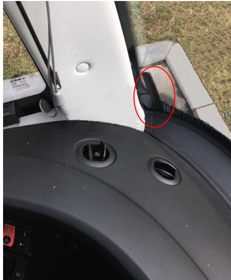
Figure 2-18 Inside installation of mobile network antenna
