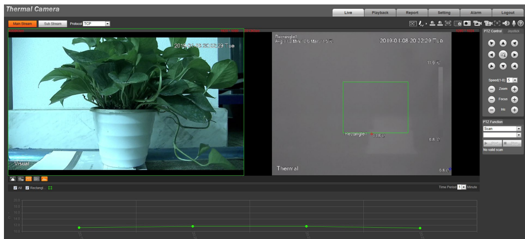
Figure 4-5 Temperature recording area
